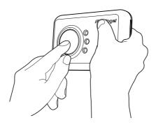
Cover the sounder vents with one hand. Press and hold the Test/Reset button down with your thumb/finger until the Fault LED illuminates amber and the sounder sounds for a second time (this should happen after around 5 seconds). Release the Test/Reset button. Upon releasing the Test/Reset button the Fault LED will flash amber once every second. This indicates that the sampling rate of the detector has increased and can be tested using a known source of CO.
